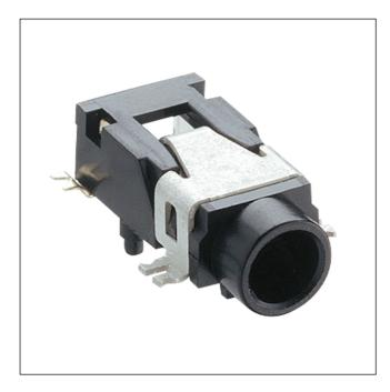
Jack chassis socket acc. to JIS C 6560 JC35J3A, 3.5 mm, 3 poles/stereo, angular version, for printed circuit boards, surface mounting technology (SMT), manual soldering only
